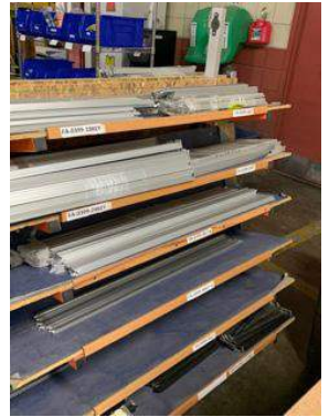
Photos from the Kaizen: the first four are “before”: three show excess inventory, the fourth (rods in trash) shows poor disposal; the final three show “after”: cleared floor, bins and racks labeled for component parts, and aluminum cut pieces labeled and organized.
